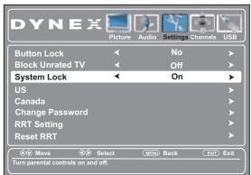
5 Press ▲ or ▼ to highlight System Lock, then press ◀ or ▶ to select On (To enable System Lock), or Off (to disable System Lock).
